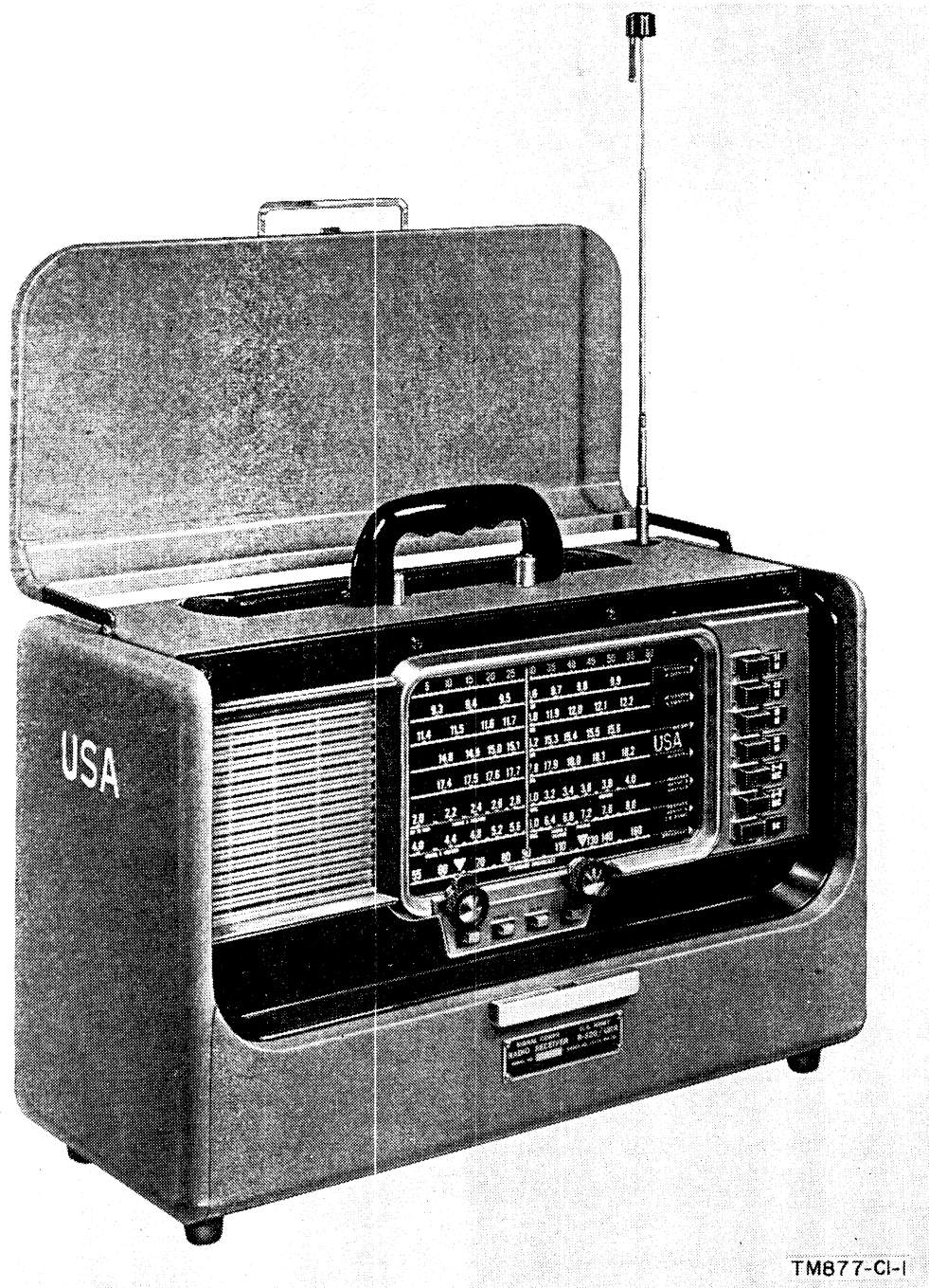
Figure 1.1. Radio Receiver R-520A/URR.
